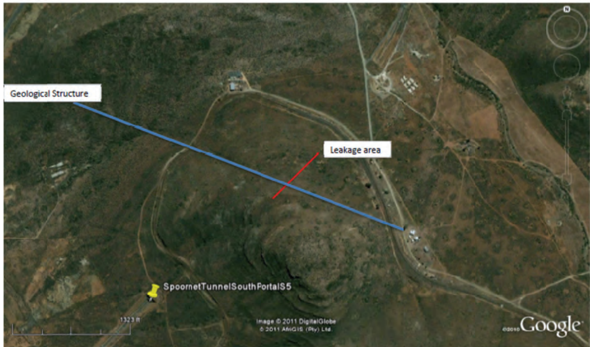
Map 5: Locality of a linear structure cutting through the tunnel at the point of seepage.
