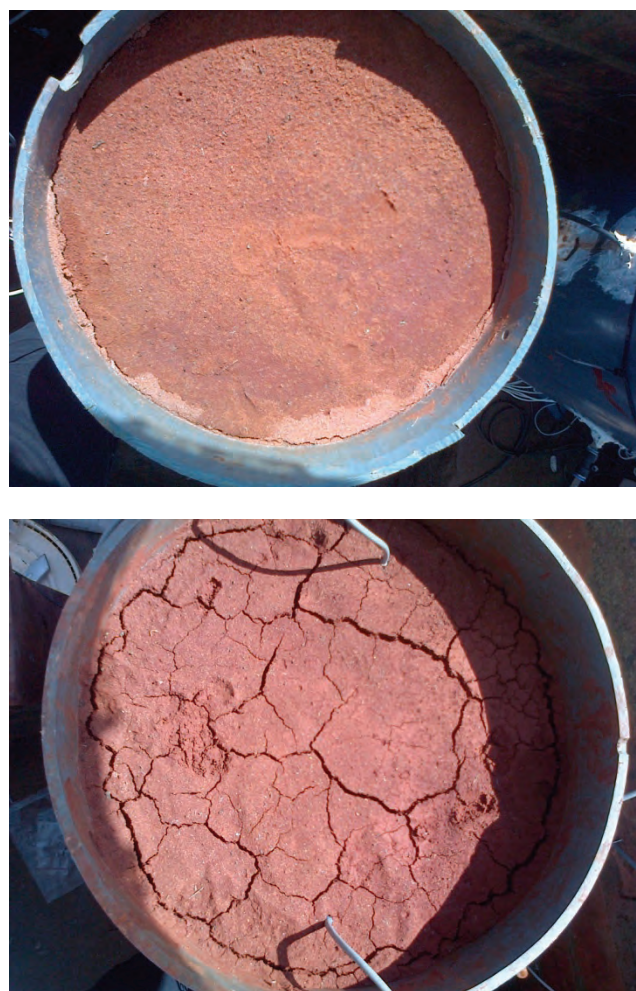
Figure 24: Columns showing the top of the slimes material (top) and sand material (bottom) after one week of evaporation.
